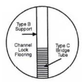
**700C Bridge Tubes** – Used with large unloading equipment
